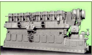
At the right is a photograph of a turbocharged version of the Cooper Bessemer Type LS marine engine.
